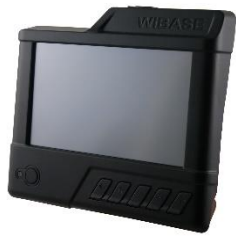
FPDLINK Display-out for WiBase Display. LCD1 – 4.3" Display
